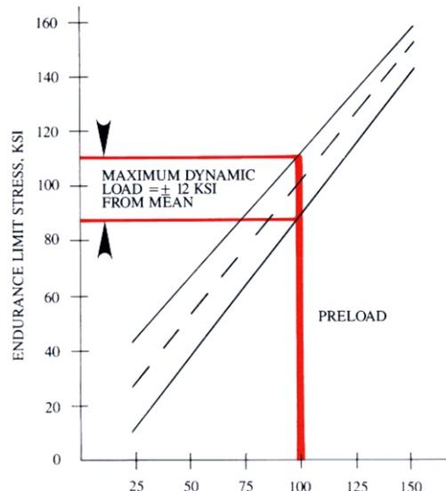
Modified Goodman diagrams help designers predict fastener performance. The broken diagonal line depicts the mean of the alternating load for a screw with a 90% probability of enduring 10 million cycles. The diagonal solid lines show that the maximum deviation of dynamic load from the mean stress is  $\pm 12$  ksi when the screw is pre-loaded to 100 ksi.
